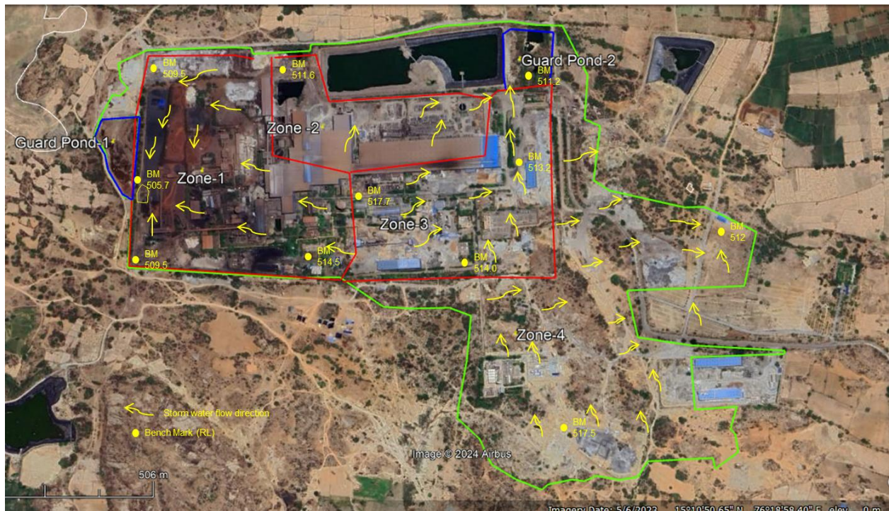
Fig. 2: Topo sheet map showing Flat terrain with small mounds at center and no drains/nalla's and TB Dam HFL on west boundary
